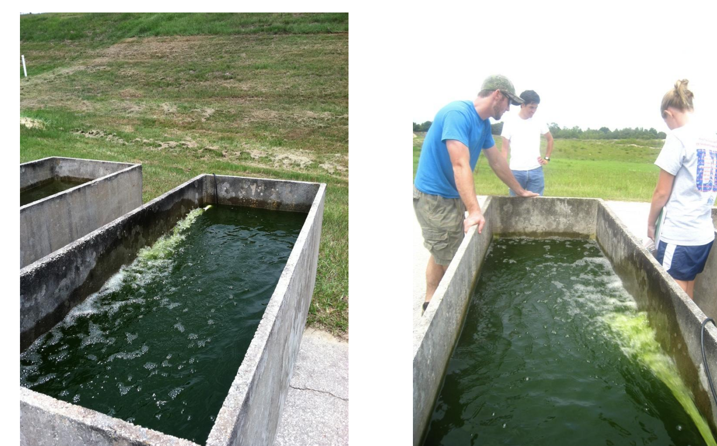
Figure 5 and 6: Algal growth in impeller-mixed, 800L algal growth chamber
