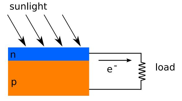
Photons striking the surface of the cell dislodge electrons.
