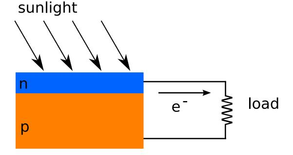
Like large area photodiodes. A diode is a solid state junction of n-type and p-type semiconductors.
