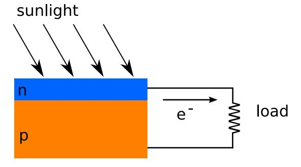
An electric field built into the diode causes electrons to accumulate on one side.
