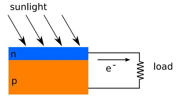
Connecting a load to the two parts of a diode causes a current to flow through it.
