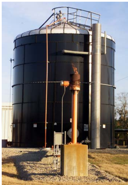
The fixed-film anaerobic digester at the UF/IFAS Dairy Research Unit produces biogas from dairy manure. Photo courtesy of Ann Wilkie
