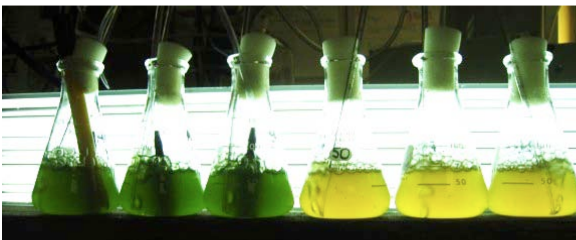
Figure 6. Cultivation of Chlorella cf. ellipsoidea in landfill leachate; triplicate cultures with pH regulation via CO 2 (left) and controls without pH regulation (right); green color correlates with algae growth and chlorophyll fluorescence at 680nm.
