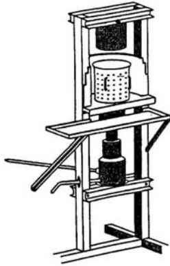
Figure 4: Hydraulic oil expeller
