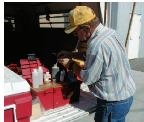
Measuring lagoon water nutrients with a nitrogen quick test
