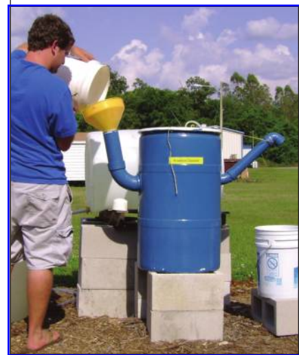
Food waste anaerobic digester.
